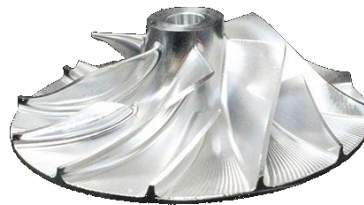
Five axis machining turbocharger impeller
