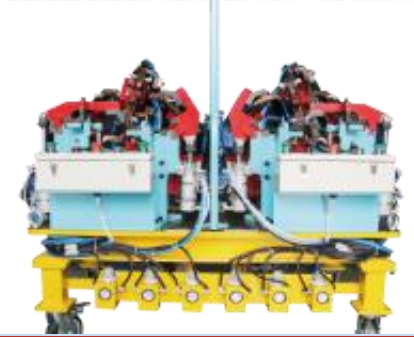
Puppet Welding jig
