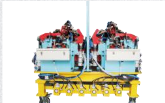
Puppet Welding jig
