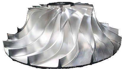
Five axis machining impeller
