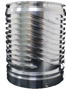
Five axis machining spiral groove
